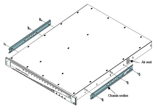
Figure B-1: Chassis section rack slides
