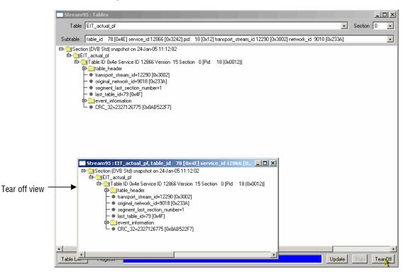
Figure 3-27: SI Tables view - Tear off view
