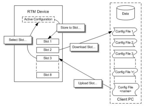
Figure 3-37: Configuration file handling
