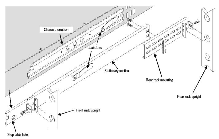
Figure B-2: Rack mounted sections
