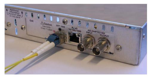
Figure B-10: SFP module - Connected
