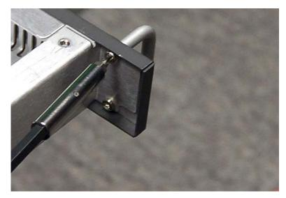
Figure B-3: Remove handle-retaining screw
