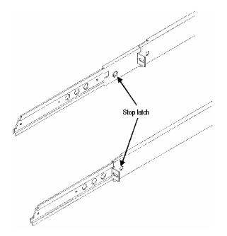
Figure B-6: Installing or removing the rack slides
