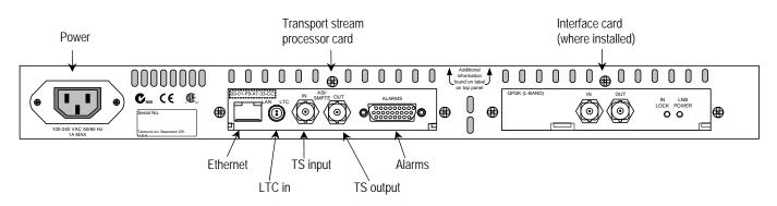
Figure 1-1: MTM400 connectors (shown with QPSK interface)
