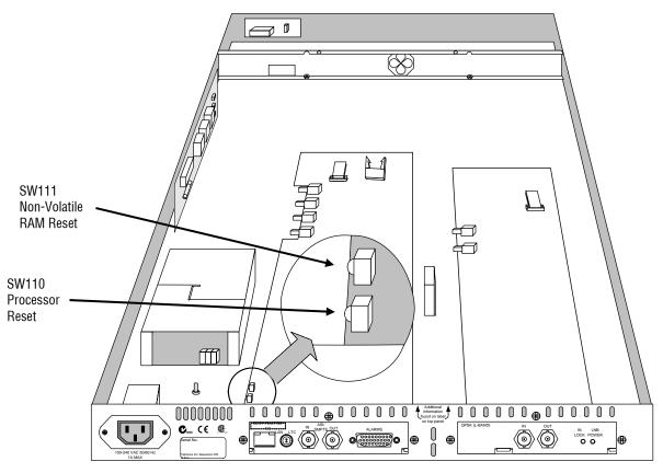
Figure A-2: Transport stream processor reset switches
